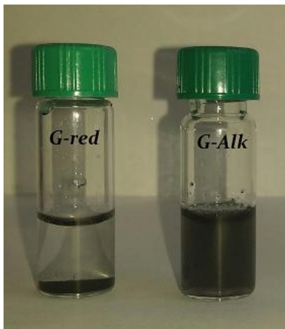
Fig.S3 Photographs of G-red and G-Alk dispersed in water ( 2 mg/mL) three days after preparation.
