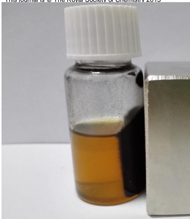
Fig. S2 Photographs of the catalyst sample separated from reactor residues under an external magnetic field.
