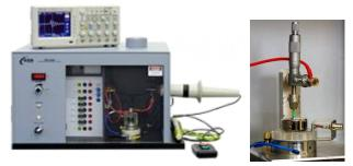
Compounds were tested for the sensitivity towards electrical discharge using an OZM Electric Spark Tester ESD 2010 EN according to STANAG 4515 instructions.<sup>8</sup> Approximately 0.1 mL volume of a compound was incorporated in a plastic tube and a charge is exerted through a steel electrode. The test is positive when a small hole was observed after the electricity interacted with the compound.
