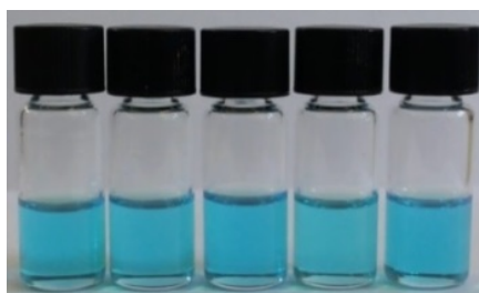
Figure S3: Chromogenic response of SQ/malaoxon (0.08 mM) complex with metal ions such as mercury (II) (0.1 mM), cadmium (II) (0.1 mM), nickel (II) (0.3 mM), copper (II) (0.3 mM) and silver ion (I) (0.2 mM).
