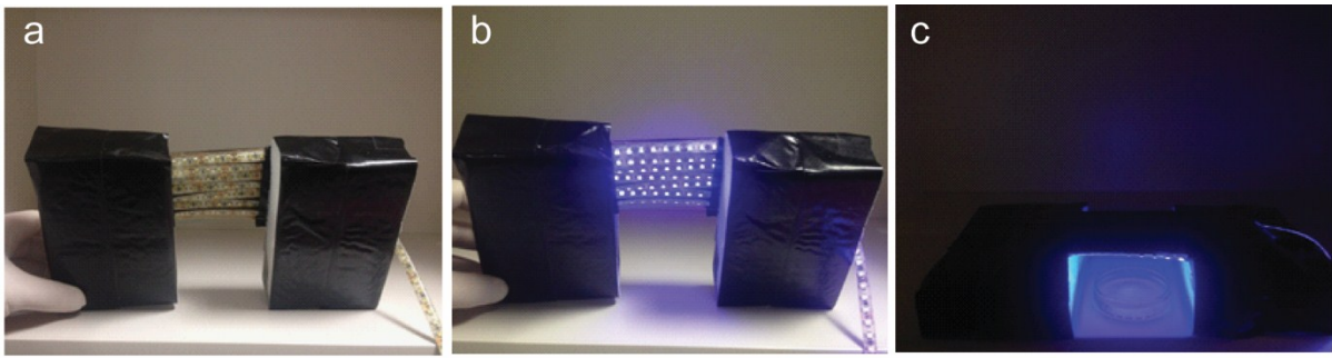
Fig. S1 a-b) Images of the ‘OFF/ON’ LED UV activation apparatus. c) The thiol-ene click reaction set in dark under UV exposure.
