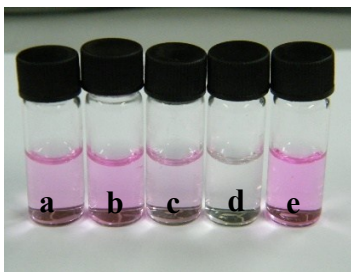
Figure S7 (a)-(d) are photodegradation results of Rhodamine B which corresponding to the (a)-(d) of Figure 4 in the text. (e) the solution before illumination.
