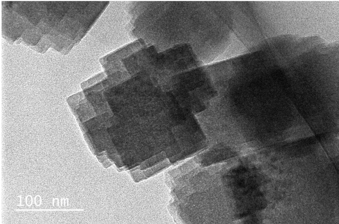
Fig. S1 Higher magnified TEM image of PB mesocrystals. Nanocubic subunits can be observed in each particle.
