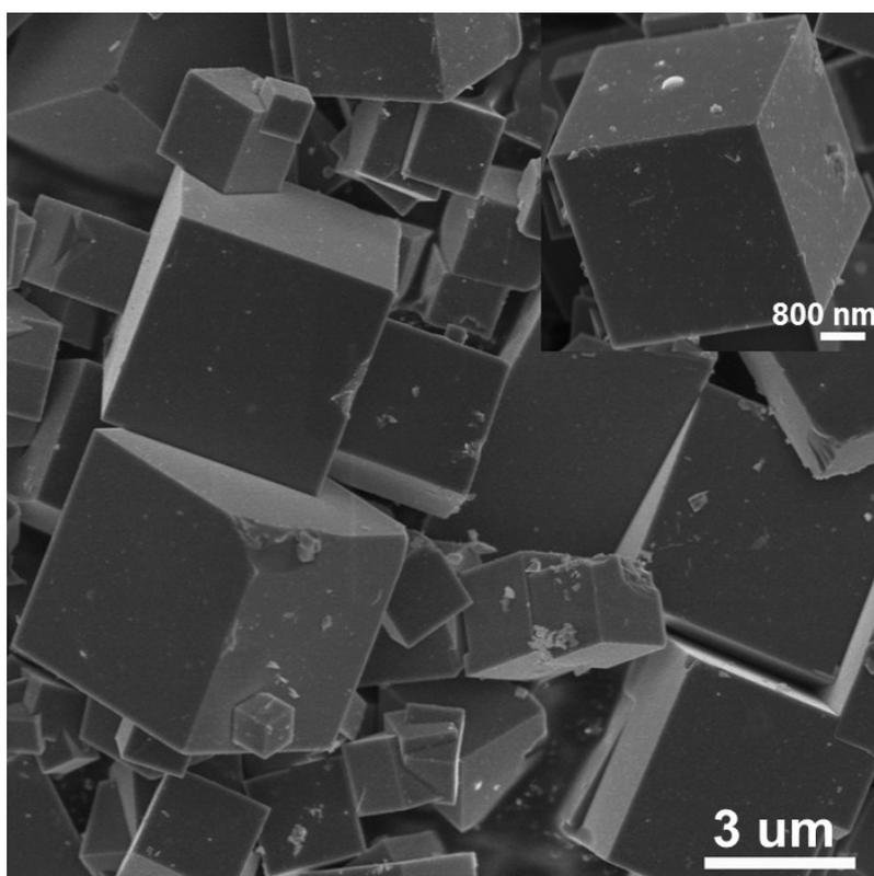
Fig. S4 SEM image of PB obtained without using PAH. The inset is a single particle.
