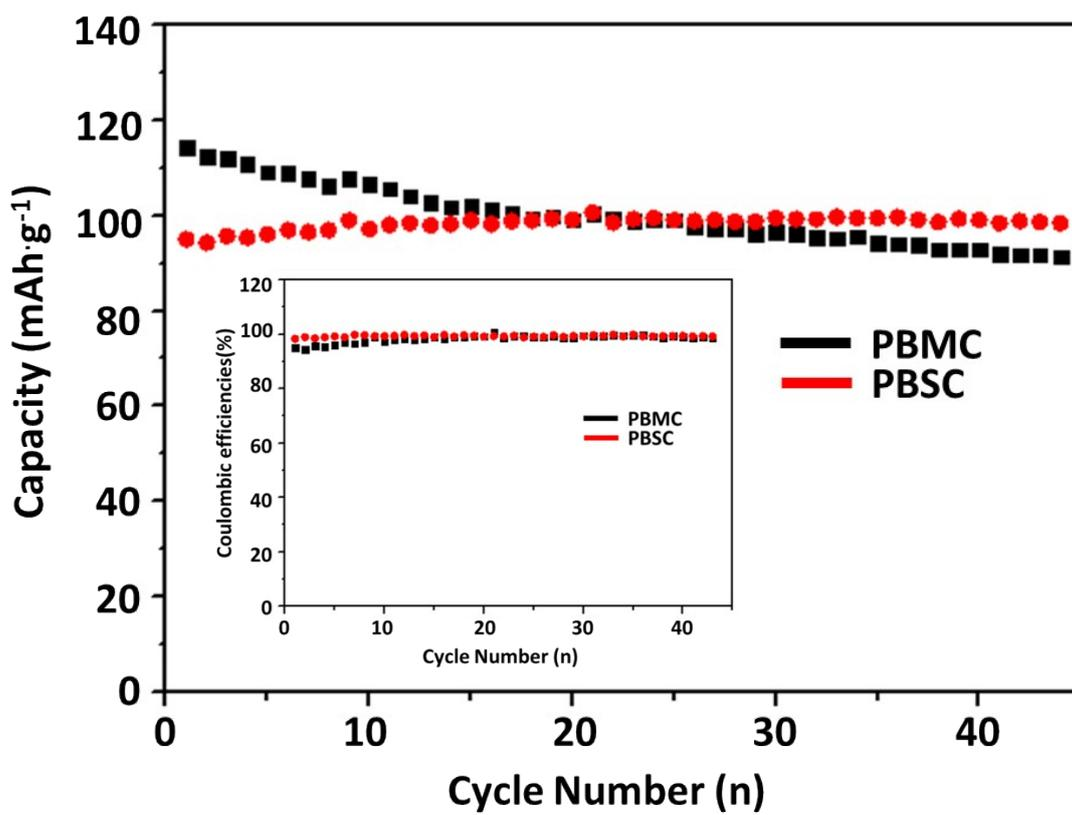
Fig. S5 Cycling performance of PB mesocrystals and single-crystals under a current density of 25 mA·g<sup>-1</sup>.
