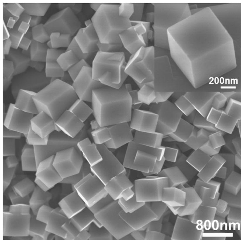
Fig. S3 SEM image of PB single-crystals. The inset is an enlarged image.
