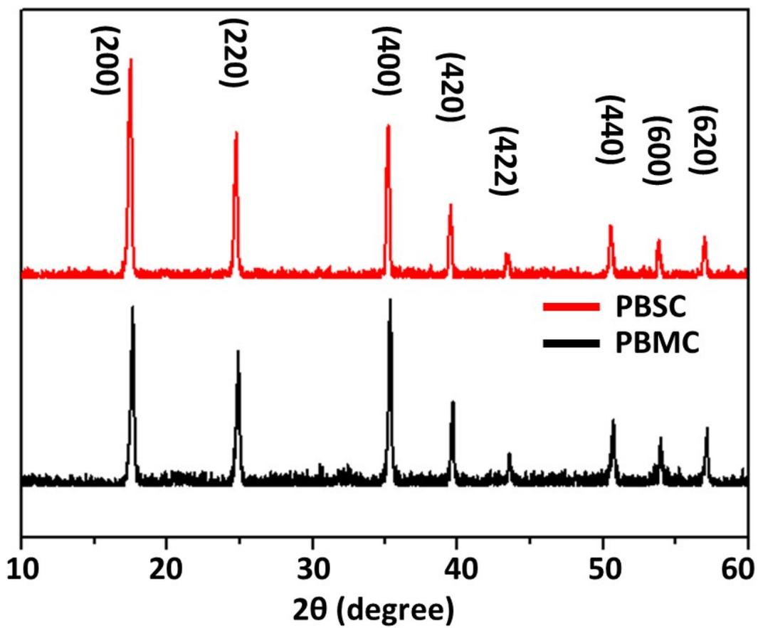
Fig. S2 XRD patterns of PB mesocrystals and single-crystals. PBSC represents PB single-crystals, and PBMC represents PB mesocrystals.
