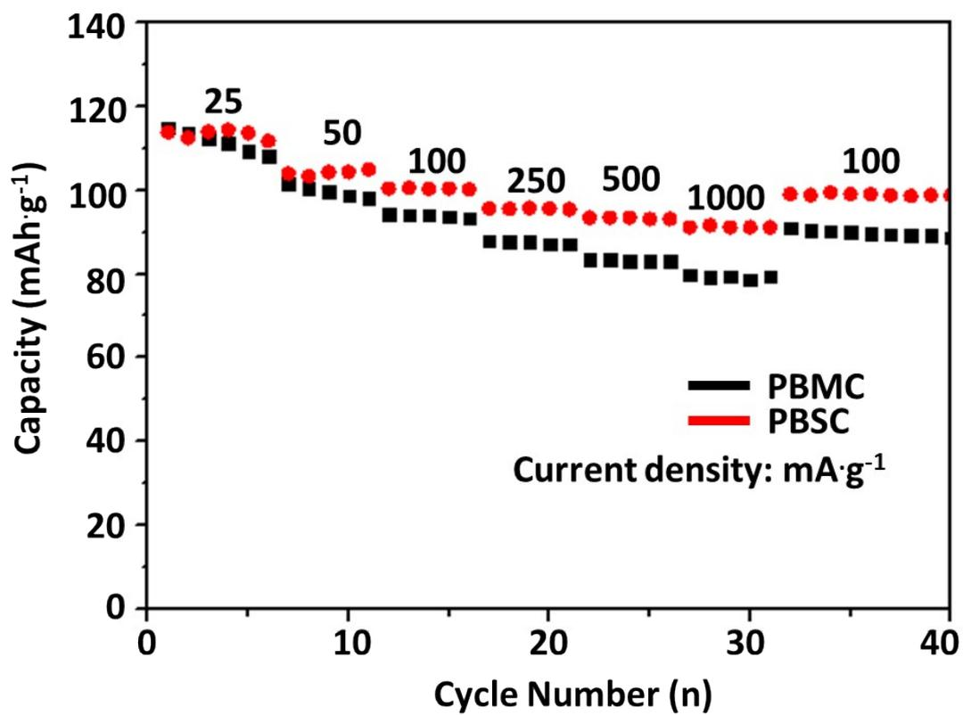
Fig. S6 Rate-performance of PB mesocrystals and PB single-crystals as cathodes for sodium ion battery.
