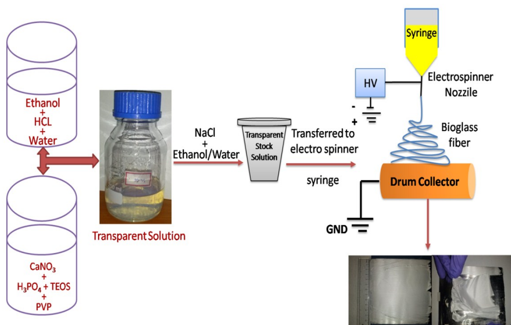
Figure S1. Schematic representation of the fabrication of Bioglass fibers using the electrospinning technique. The Bioglass containing transparent solution has been diluted with ethanol or water and fed to the electrospinning setup. The high voltage power leads to the formation of fibers and it was collected using a drum collector.
