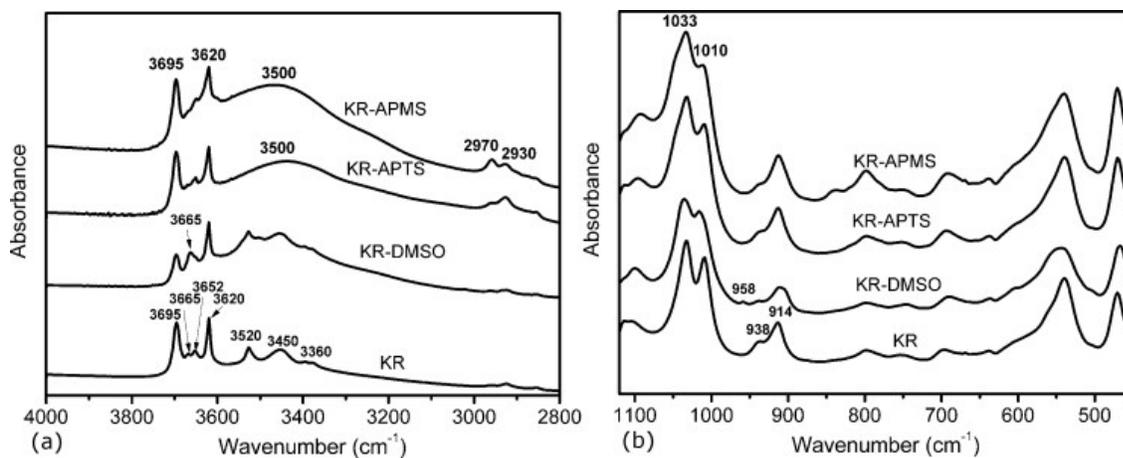
Figure S8. The infrared spectra of KR, KR-DMSO, KR-APTS and KR-APMS in the 4000-2800  $\text{cm}^{-1}$  (a) and 1100-450  $\text{cm}^{-1}$  (b) specific wavenumber range
