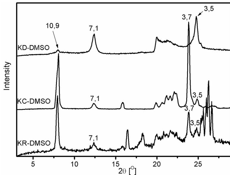
Fig S7. XRD patterns of the three DMSO-intercalated kaolin samples
