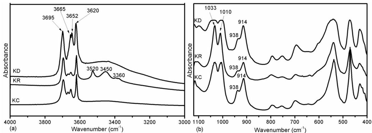
Fig S3. Infrared spectra of the three kaolin samples; (4000-3000 $cm^{-1}$ ) (a) and (1150 – 450  $cm^{-1}$ ) (b) wavenumber ranges
