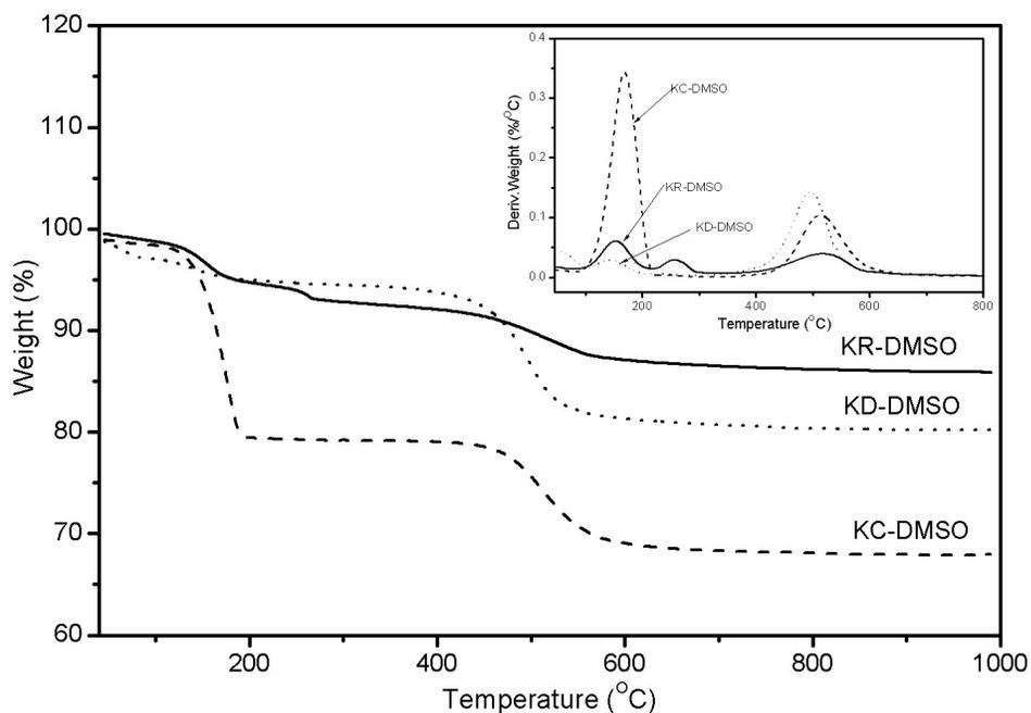
**Fig S5.** The TGA curves /DTG inset of the three DMSO-intercalated kaolin samples
