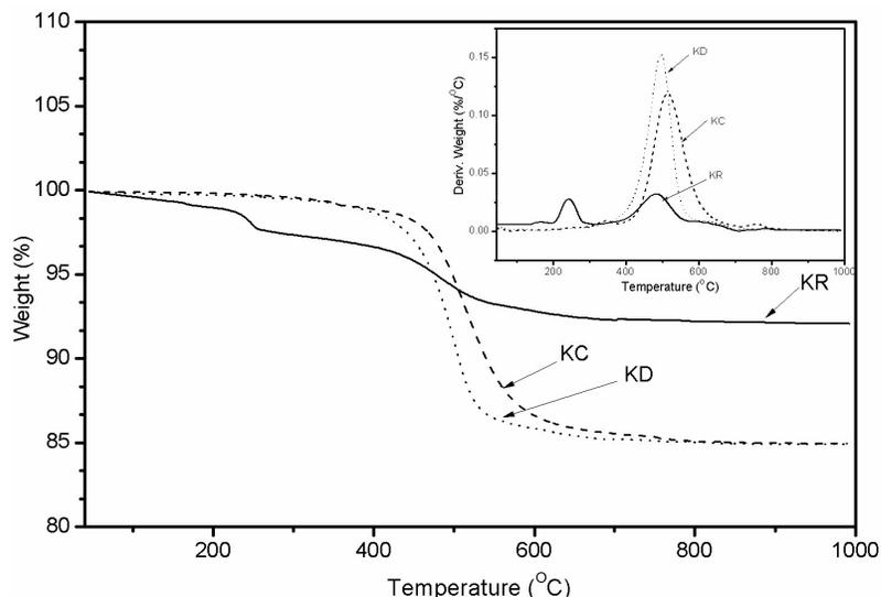
Fig S2 TGA curves/DTG inset of the three kaolin samples
