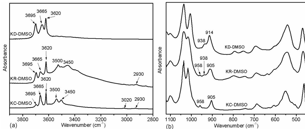
**Fig S6.** Infrared spectra of the three DMSO-intercalated kaolin samples; (4000-3000 $\text{cm}^{-1}$ ) **(a)** and (1150 – 450  $\text{cm}^{-1}$ ) **(b)** wavenumber ranges
