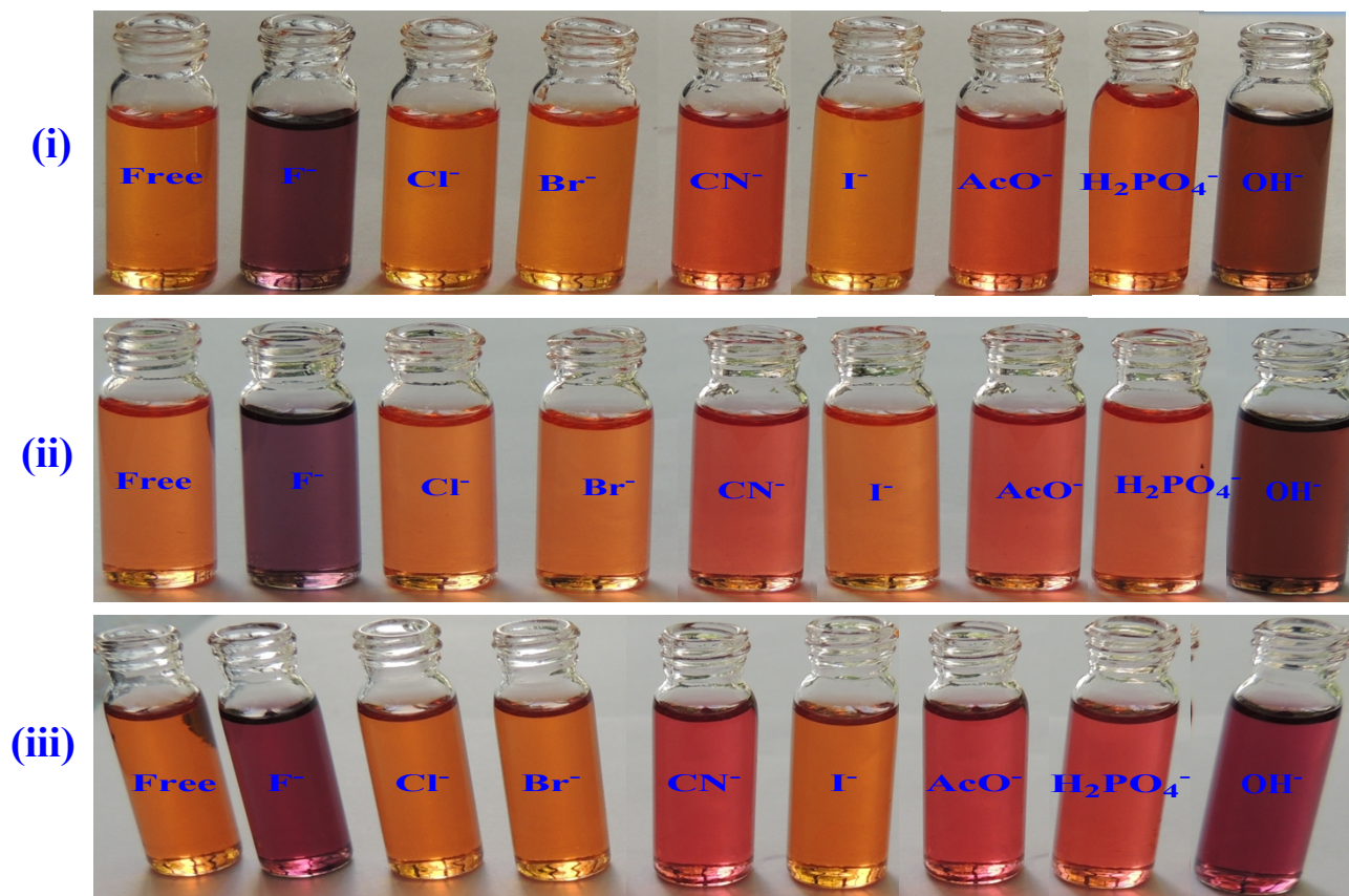
Fig. S2 Color changes that observed when the DMSO solutions of 1 (i), 2 (ii) and 3 (iii) are treated with different anions as their tetrabutylammonium (TBA) salts.
