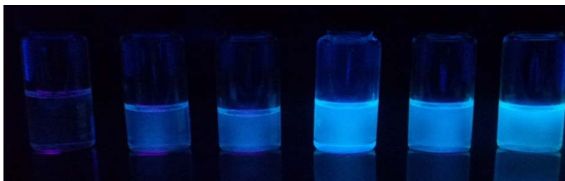
Fig. S1 The reactant colour changed over time under ultraviolet (UV) irradiation at 365 nm (from left to right 0, 2, 5, 10, 15, 20min).
