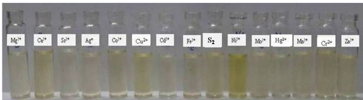
ESI Fig. 1 Visual ion sensing of S_1 and S_2 with various metal ions in DMF.
