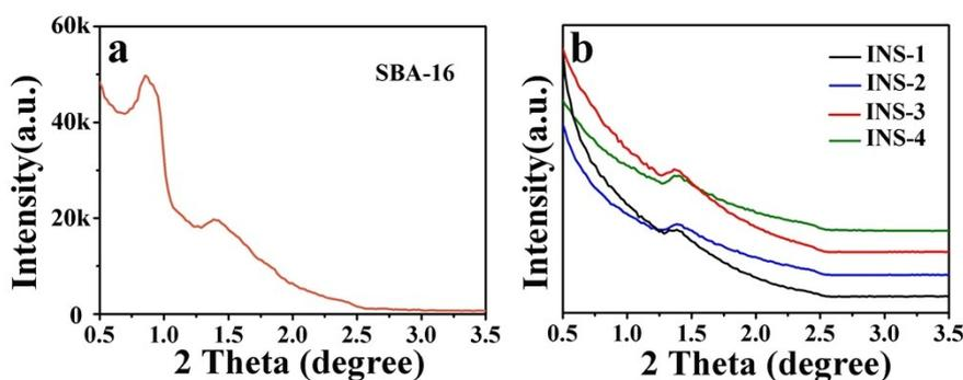
Fig. S1 Low-angle XRD X-ray diffraction diagrams of SBA-16 (1) and mesoporous In<sub>2</sub>O<sub>3</sub> materials replicated from mesoporous silica of INS-1, INS-2, INS-3, INS-4. respectively.
