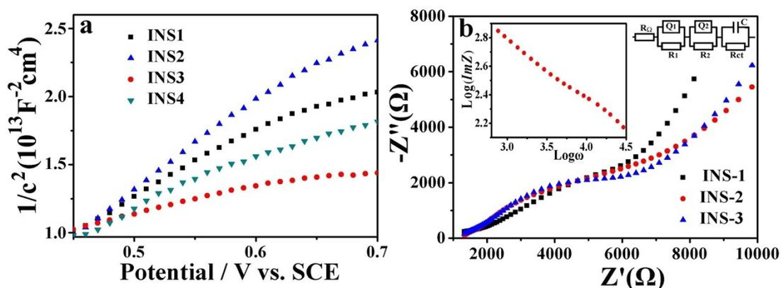
Fig. S4 (a) The Mott-Schottky curves of INS-1, INS-2, INS-3 and INS-4 samples, (b) The EIS curves of INS-1, INS-2 and INS-3 samples. The right inset is the corresponding equivalent circuit model, the inset in left shows the logarithmic plot of the imaginary part of the impedance.
