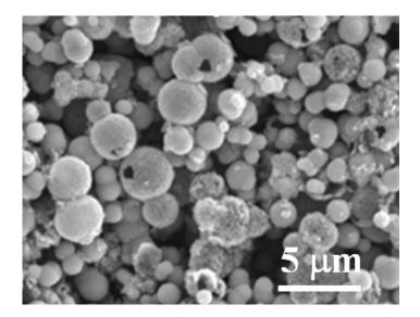
Fig. S1 SEM image of NiS hollow microspheres.
