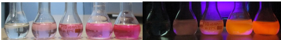
Fig. S11: Change in colour in the solution of 1 (2 × 10 -5 M) in MeCN-H 2 O (1:1 v/v, pH 7.2) upon addition of 0, 1, 2, 3 and 5 eq. of Hg 2+ under (a) normal light and (b) upon irradiation at 450 nm.
