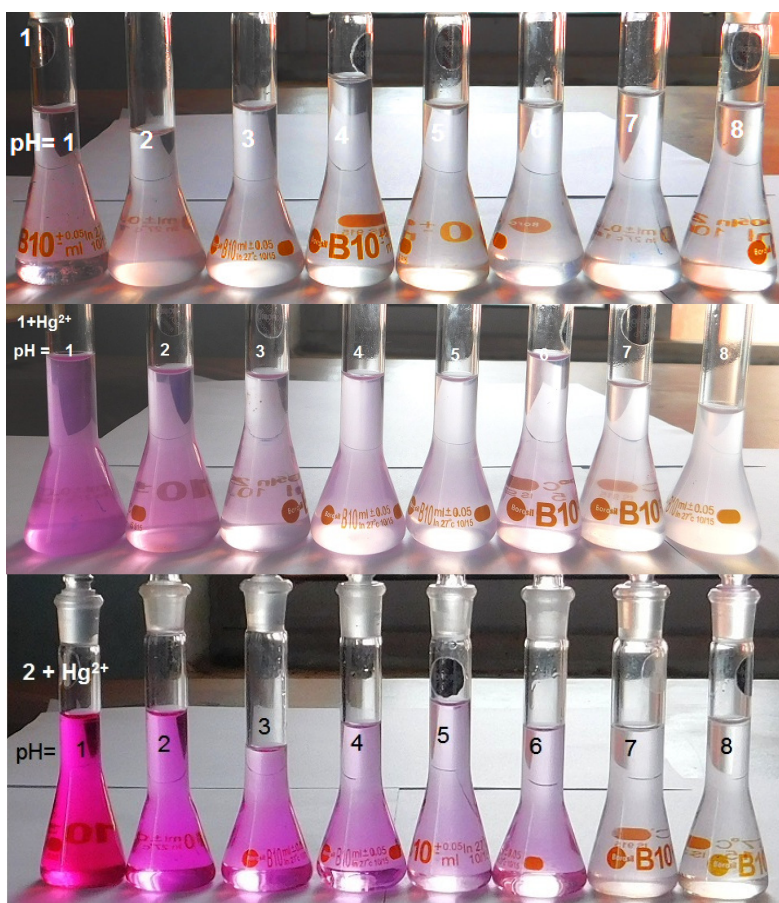
Fig. S32: Colorimetric mapping of (a) 1 alone, (b) 1 +Hg 2+ and (c) 2 +Hg 2+ in MeCN-H 2 O (1:9 v/v, PBS buffer) under different pH (pH = 1-8) conditions. [ 1 or 2 ] = 10 μM.
