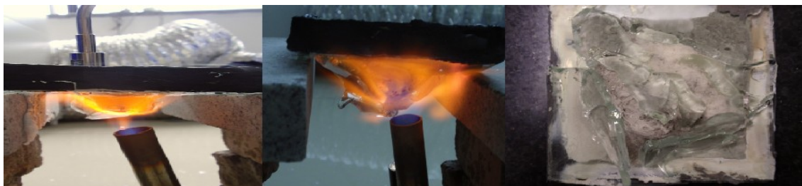
Figure S3 Fire resistant glazing during the fire test (Formula 3)
