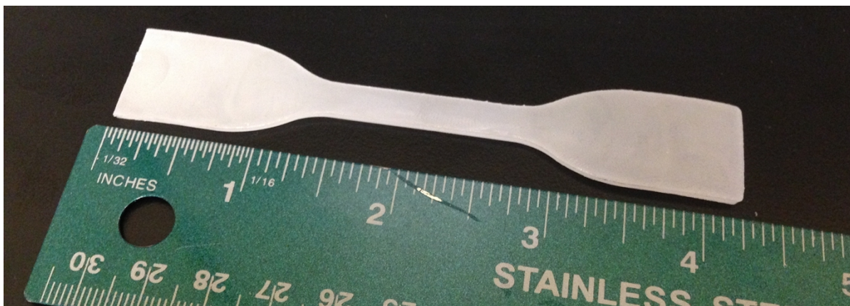
Figure S2: An ASTM Type IV dog-bone sample was molded to demonstrate the ability to manufacture large LCE samples.
