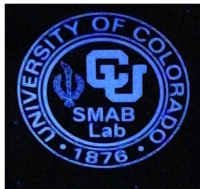
Figure S5: Image of an LCE sample being covered with a photo-mask and exposed to UV light to spatially control the second-stage photo-crosslinking reaction.
