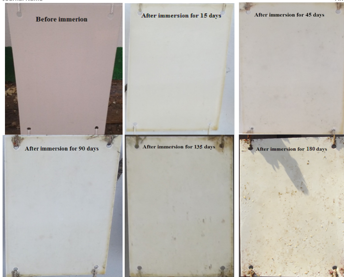
Figure S6: Field test of PDMS/Cu 2 O nanocomposites for 6 months of immersion.
