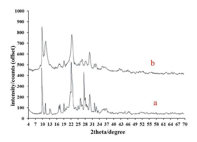
Figure. 2s. XRD pattern of Cu-ZSM-5 (a), RGO/Cu-ZSM-5 (b).
