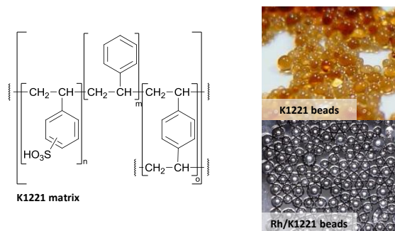
Figure S1. Chemical structure of the K1221 ionic exchange resin (left); images of the parent K1221 beads (top right) and of the Rh/K1221 beads after immobilization of the metal nanoparticles (bottom right).
