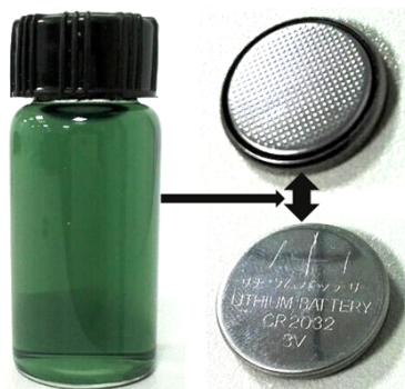
Fig. S1 The two-electrode CR2032-type coin cells assembled by the result green products.
