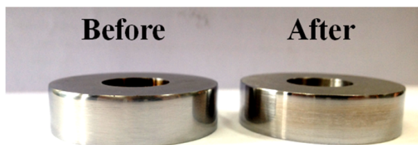
Fig. S13 Digital photos of counterpart steel ring friction before (a) and after (b) the friction tests of HBPT-RGO/BMI-BA composite.
