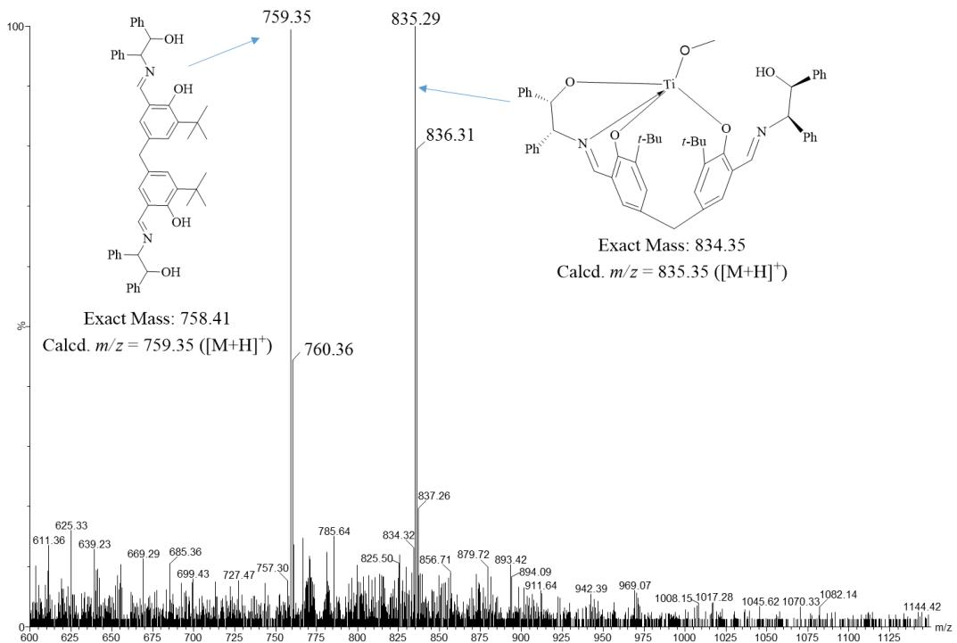
**(b) ESI-MS analysis of *in situ* generated **L1-Ti** complex at **L1:Ti = 1:2**.**
