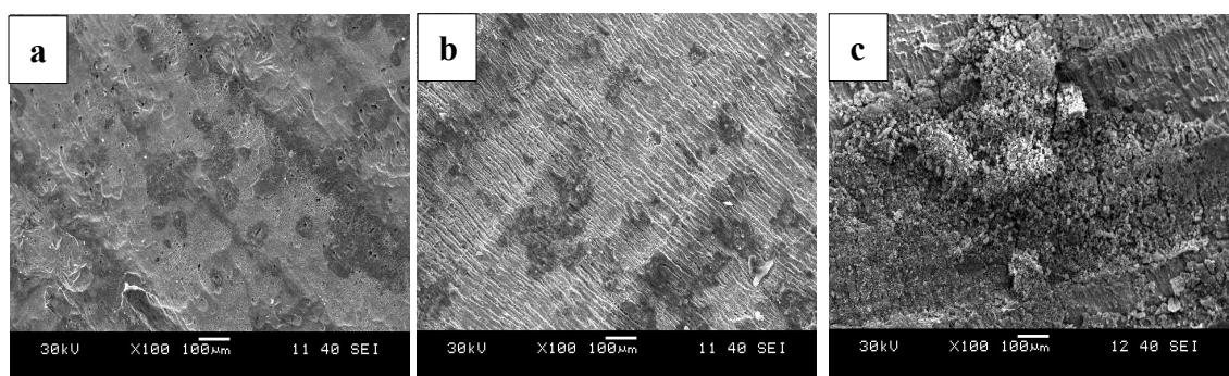
**Fig.S1** SEM images of fresh ZVI (a), ZVI shavings after reduction (b) and ZVI shavings after oxidation (c)
