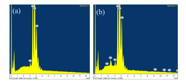
Figure S3 The EDS results for (a) SnTe and (b)  $SnPb_{0.02}Te$ . The peak for Pb is clearly observed in (b). (c) Composition distribution of ten different parts of  $SnPb_{0.02}Te$ .
