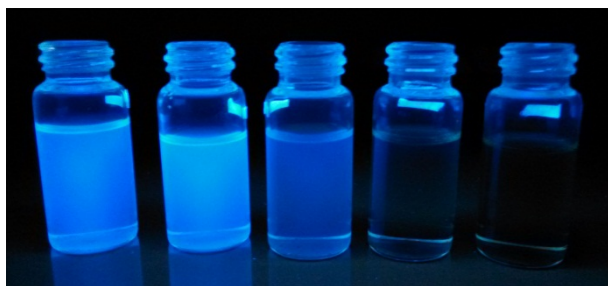
Fig. S5 Optical images of the samples in \text{Cu}(\text{NO}_3)_2 DMF solutions at different concentrations (left to right: 10^{-6} mol/L, 10^{-5} mol/L, 10^{-4} mol/L, 10^{-3} mol/L, 10^{-2} mol/L) under 365 nm UV light irradiation.
