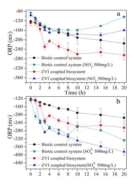
**Figure S3** Evolution of the ORP during the reduction of DNAN in the two individual systems with the coexistence of different electron acceptors: (a) nitrate; (b) sulfate.
