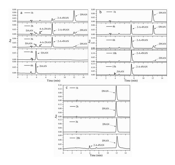
**Figure S1** Evolution of HPLC chromatogram for the DNAN reduction in three individual systems as a function of time: (a) ZVI coupled anaerobic system; (b) biotic control system and (c) ZVI control system.
