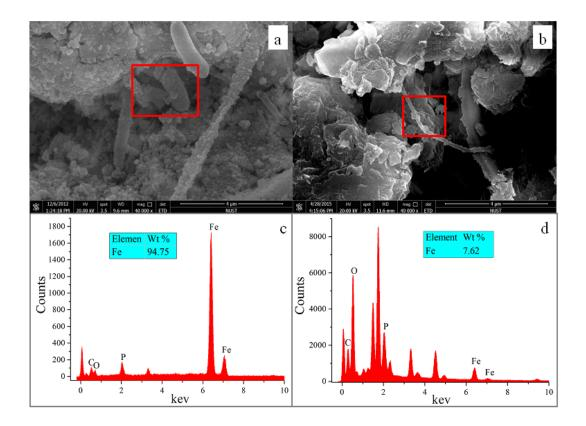
**Figure S2** SEM images showing the morphology and distribution of ZVI on the outer layer (a) and inner parts of the microorganisms (b); EDS spectrums for the selected area of the SEM image a(c) and image c(d).
