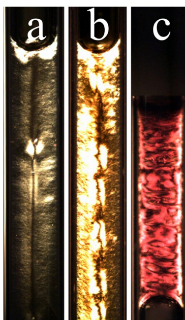
Fig. S8 POM images of GO aqueous dispersions at the same concentration for GO-1, GO-6 and GO-12 in capillaries observed between crossed polarizers.
