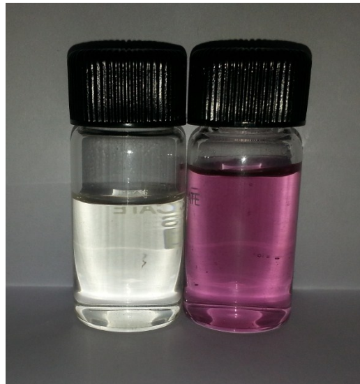
Figure S2: Colour change of N1 on formation of H1 from colourless to pink
