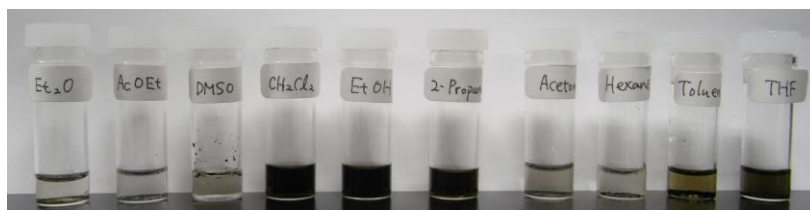
Fig. S2 Pictures of PMAP-DDDMA (a) before and (b) after washing in various solvents (from left to right, diethyl ether, ethyl acetate, DMSO, CH_2Cl_2 , ethanol, 2-propanol, acetone, hexane, toluene and THF ).
