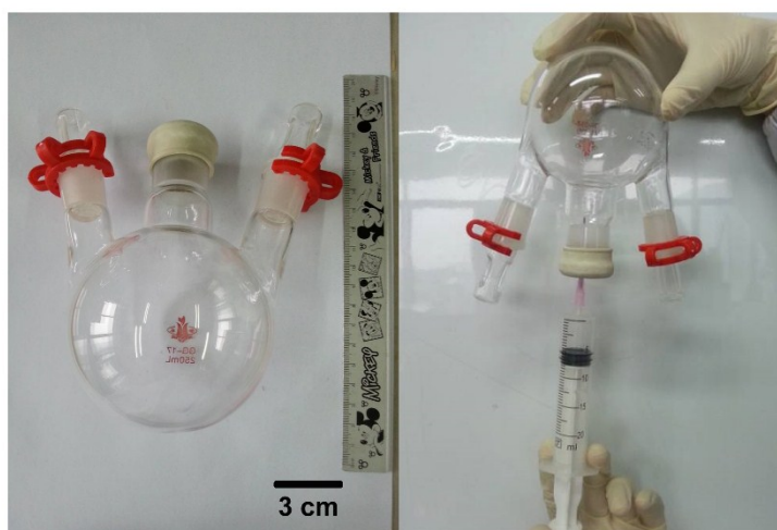
Figure S10. Procedure of injecting the gaseous ammonia into the three-necked flask.
