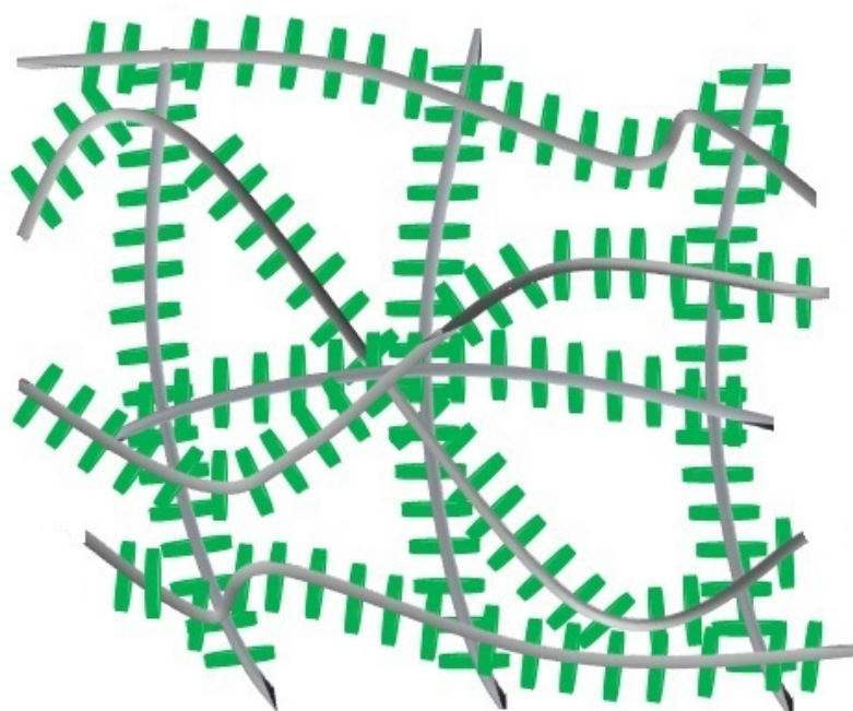
Figure S3. The schematic diagram showing how the surface formed LDH and MgCO 3 films were separated by the Al-foil substrates.
