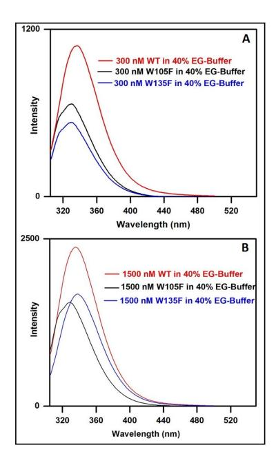
Figure S1: Steady state fuorescence spectra at 298 K of WT CHPV and the mutants W135F and W105F in 40% EG- buffer at (A) 300 nM concentration and (B) 1500 nM concentration.  $\lambda_{exc} =$  295 nm, Excitation and emission bandpass = 10 nm and 5 nm each.
