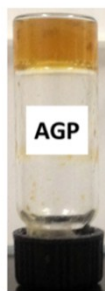
Fig. S5 Photograph of the gelation test of AGP in PBS (6.6 mg/mL).
