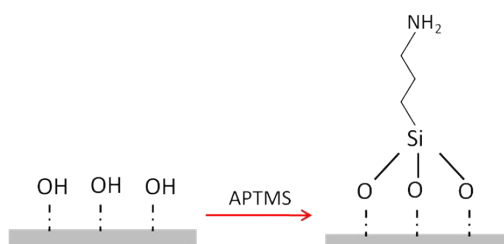
Fig. S2. Functionalization of the inner walls of AAO nanotube array with APTMS.
