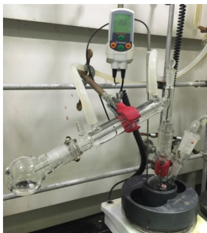
Fig. S1 The reaction flask was fitted with a distillation apparatus containing sat. sodium thiosulfate (4ml) in receiving flask
