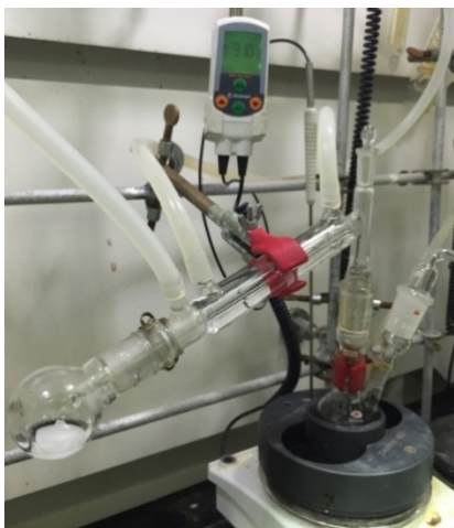
Fig. S2 HBr and Br 2 were trapped by sat. sodium thiosulfate in receiving flask
