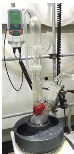
Fig. S3 The resulting solid was heated at 180 °C for 1 hour under a nitrogen atmosphere.
