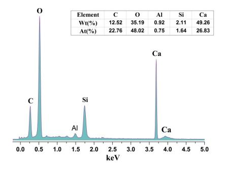
The energy dispersive X-ray spectroscopy of the oyster shell powder
