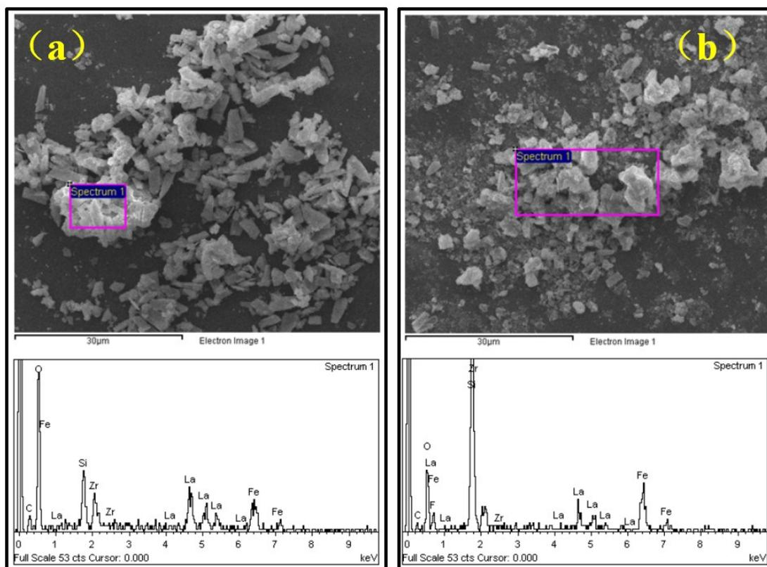
Fig. S2. (a) EDS of La-Zr magnetic composite; (b) EDS of La-Zr magnetic composite dried at 60°C after adsorbed 300 mg/L F<sup>-</sup>.
