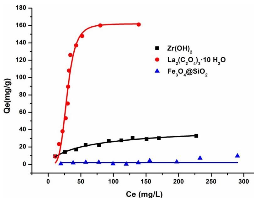
Fig. S3. Comparison between the measured and Lan-Fre isotherm modeled profiles of  $\text{ZrO}(\text{OH})_2$ ,  $\text{La}_2(\text{C}_2\text{O}_4)_3 \cdot 10 \text{H}_2\text{O}$  and  $\text{Fe}_3\text{O}_4@\text{SiO}_2$ .
