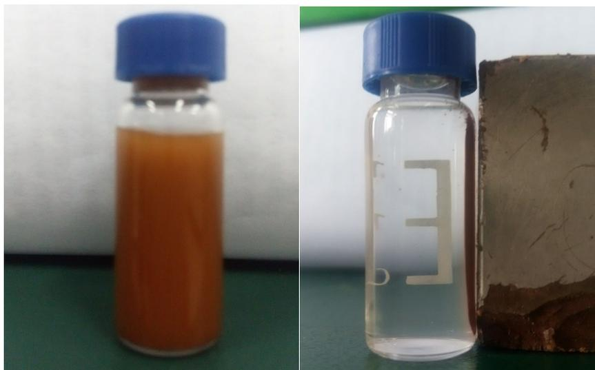
Fig. S1. The composite in the absence (left) and presence (right) of an external magnetic field
