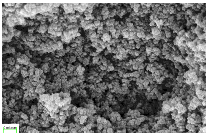
Figure S1. SEM image of MM6 fracture surface.
