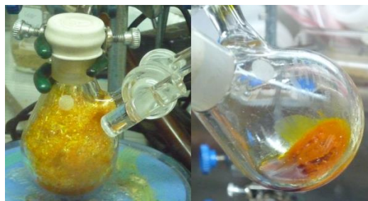
Figure S1. Left: Foam-like 10-Ir-HBpin ; Right: 10-Ir-HBpin after recrystallization from hexamethyldisiloxane.
