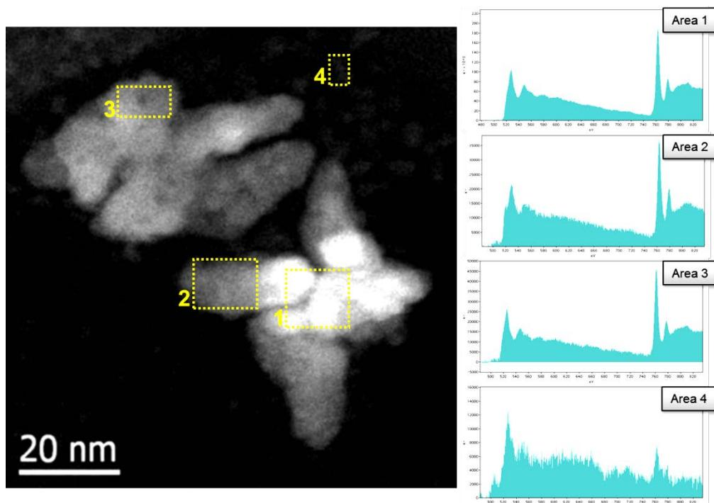
**SI 5:** TEM image of the CoO/FLG system illustrating a completely different morphology compared to that corresponding to the CoO/CNTs system where confinement effect operates.
