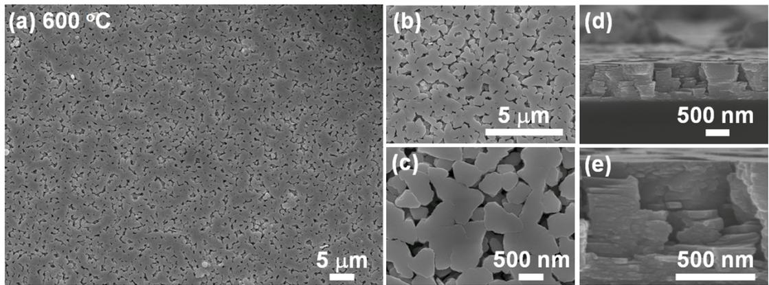
**Figure S4.** (a)-(c) The top-view SEM images clearly show numerous nanoscopic holes periodically embedded in the  $\text{Bi}_2\text{Te}_3$  superassemblies prepared at 600 °C. (d)-(e) The corresponding cross-sectional SEM images indicate that the 2-D nanoflakes are horizontally lying on the  $\text{SiO}_2/\text{Si}$  substrate.
