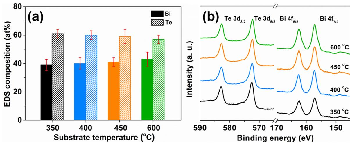
**Figure S6.** (a) The EDS compositional analyses of the Bi<sub>2</sub>Te<sub>3</sub> superassemblies fabricated at various temperatures. (b) The XPS spectra of the Bi 4f and Te 3d states evidence the absence of oxidation states.
