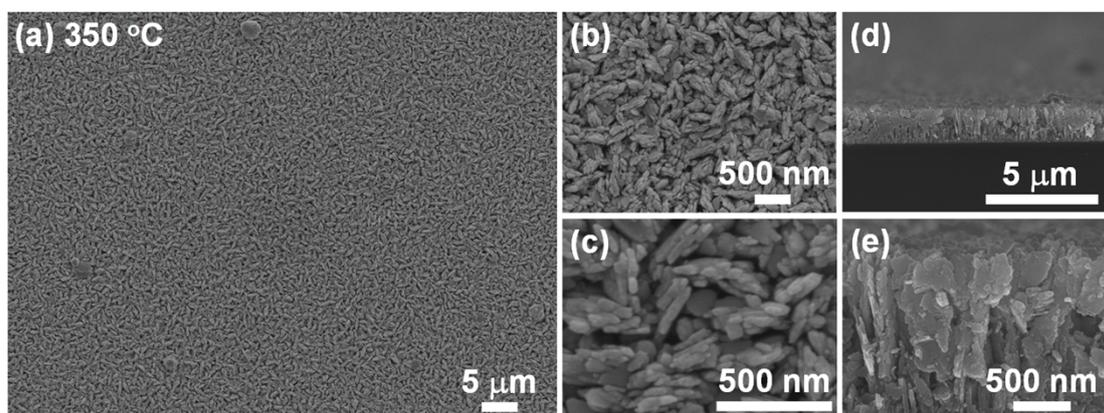
**Figure S1.** (a)-(c) The top-view SEM images indicate that the  $\text{Bi}_2\text{Te}_3$  superassemblies deposited at 350 °C are uniformly composed of spindle-like hierarchical nanostructures. (d)-(e) The cross-sectional SEM images confirm that the nanoarchitectures are vertically-aligned on the  $\text{SiO}_2/\text{Si}$  substrate.
