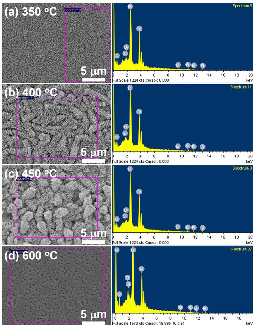
**Figure S5.** The low-magnification top-view SEM images of the  $\text{Bi}_2\text{Te}_3$  superassemblies fabricated at (a) 350 °C, (b) 400 °C, (c) 450 °C, and (d) 600 °C. The corresponding EDS spectra clearly show Bi, Te, Si, and O signals originated from the  $\text{Bi}_2\text{Te}_3$  superassemblies and  $\text{SiO}_2/\text{Si}$  substrate. This result is consistent with the XPS investigations.
