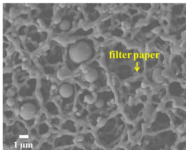
Figure S9. SEM image of PANI spheres via interfacial polymerization route. Conditions: PFOA:aniline:APS=1:1:1, PFOA=10 mM, polymerization time=20 h.
