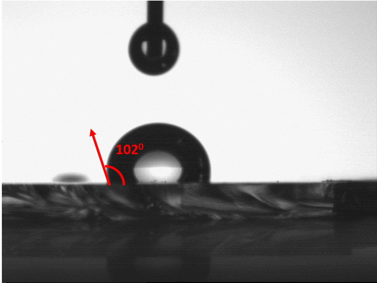
S5: Contact angle measurement of Z@C dots nanocomposite; with contact angle higher than 90° (showing hydrophobic nature of Z@C dots )
