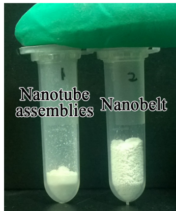
Fig. S4. Volume comparison of the \text{TiO}_2 nanotube assemblies and the \text{TiO}_2(\text{B}) nanobelts with the same mass.
