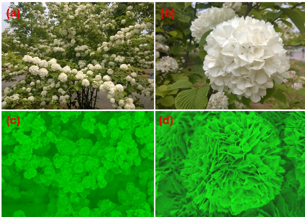
Figure S5. (a, b) Optical photographs of flowers in the real world; c, d) low-magnification and high-magnification SEM images of the \text{ZnCo}_2\text{O}_4 NFs.
