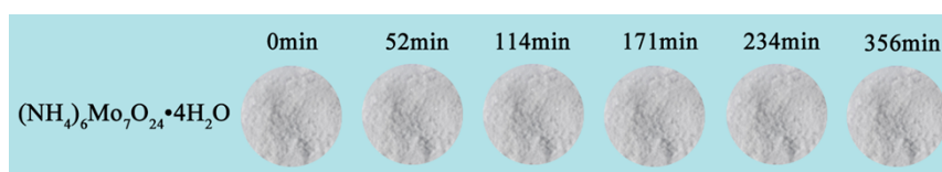
Fig. S12 Color of (\text{NH}_4)_6\text{Mo}_7\text{O}_{24}\cdot 4\text{H}_2\text{O} after certain minutes irradiation by xenon lamp.
