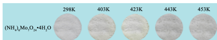
Fig. S2 Color of (NH_4)_6Mo_7O_{24} \cdot 4H_2O at different temperatures.
