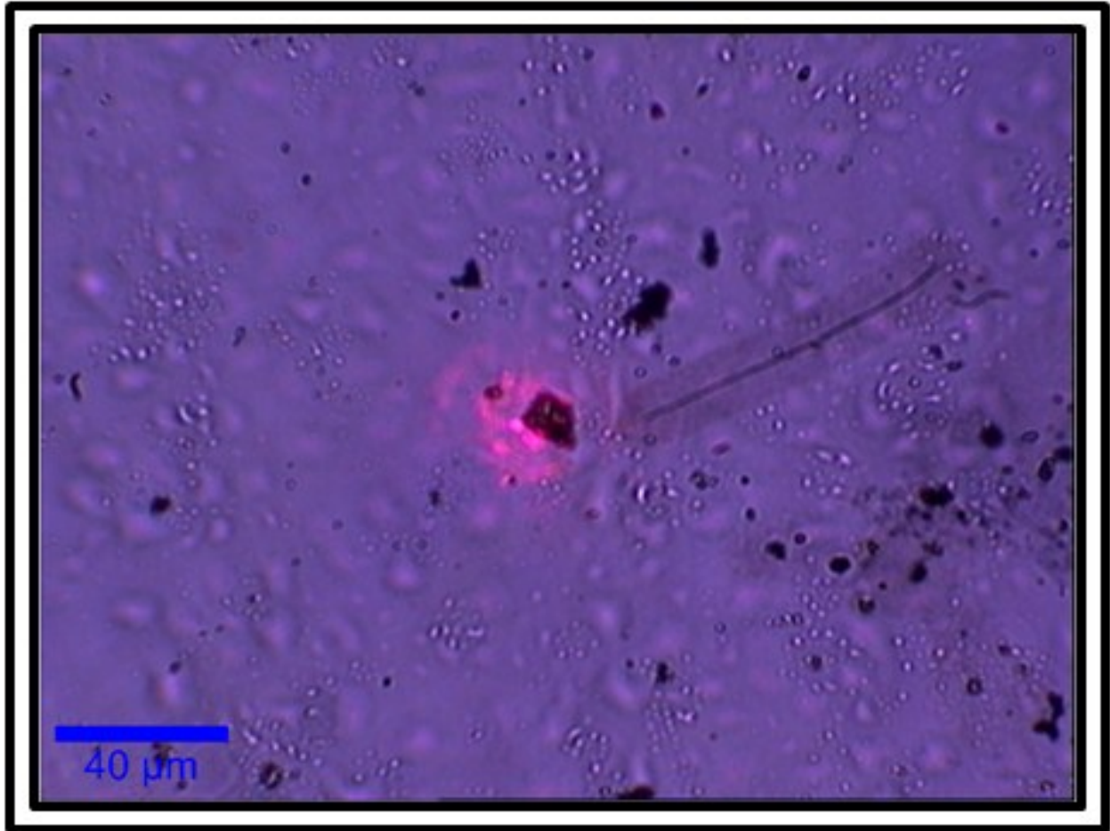
Fig. S8. Optical micrograph image of Ag/ZnS/Ag multilayer thin film; it was taken using confocal PL mapping instrument.
