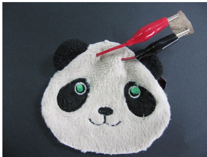
Figure S9. The LED connected with a GO-coated silk fabric.
