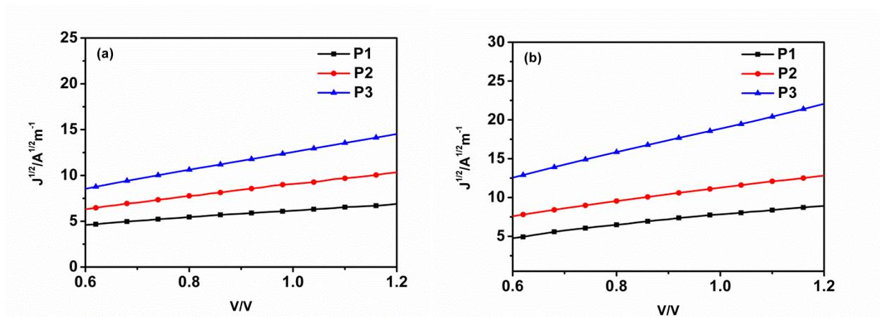
Fig. S4 Hole mobility of **P1-3**:PC<sub>71</sub>BM based devices without (a) and with 2% DIO (b) by SCLC.
